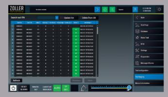
»micBox« database overview – provides a reliable overview of all relevant information of the currently loaded tool, such as how many indexable inserts have been used and how often an exchange has already taken place.
