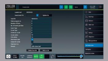
»micBox« tool configuration – simple and efficient, new tools can be created quickly and necessary information for the robot entered. Existing tools can also be edited and updated at any time.
