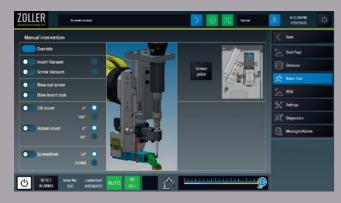
»micBox« user interface – offers a clear overview of all available modules – from robot control to turning and rotating unit to the lubrication station for screws. Each module can be conveniently operated manually, including the robot directly via the software.
