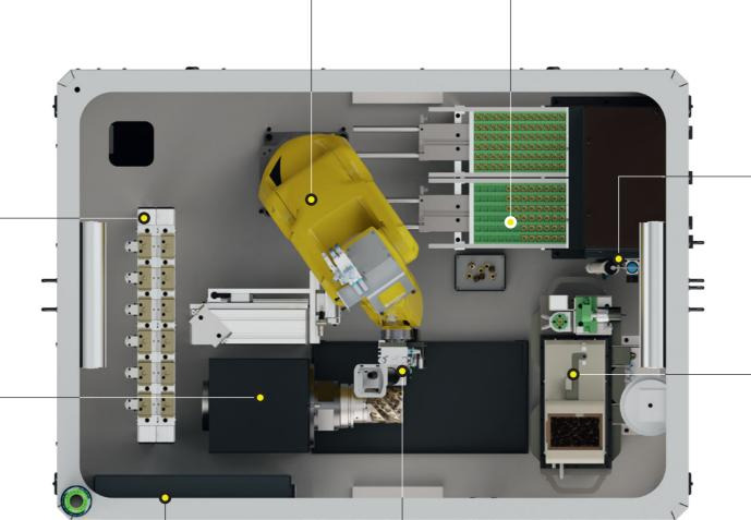
Magazine for indexable inserts – provides sufficient space. The two magazines inside the »micBox« can be stocked differently.
